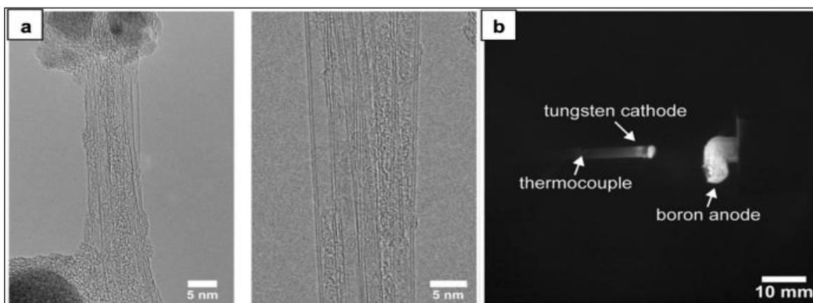
(a) Single and double-walled BNNT synthesised by arc discharge method; and (b) IR image of the cathode and anode electrodes in the chamber. Source: Y.-W. Yeh et al., Stable synthesis of few-layered boron nitride nanotubes by anodic arc discharge. *Sci. Rep.* 7(1), 3075 (2017)
