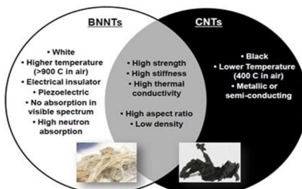
BNNT vs CNT comparison, Source: Boron Nitride Nanotubes: Properties, Synthesis and Applications, Richard Dolbec, Sigma Aldrich
