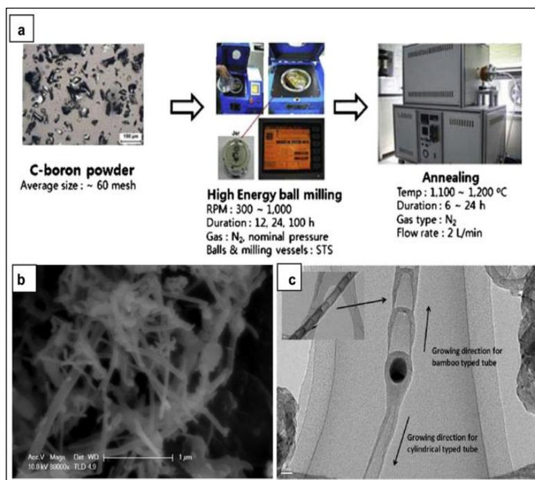
(a) Experimental procedure of ball-milling method. (b) SEM and (c) TEM image of BNNTs produced by the ball-milling method. Cylindrical- and bamboo-like shape of BNNTs is shown in TEM image. Source: J. Kim et al., Synthesis and growth of boron nitride nanotubes by a ball milling-annealing process. Acta Mater. 59(7), 2807-2813 (2011)
