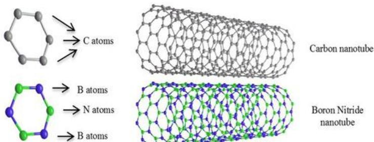
Structure of BNNTs vs CNTs. Source: Comparison of small scale effect theories for buckling analysis of nanobeams, Kadir Mercan & Omer Civalek
