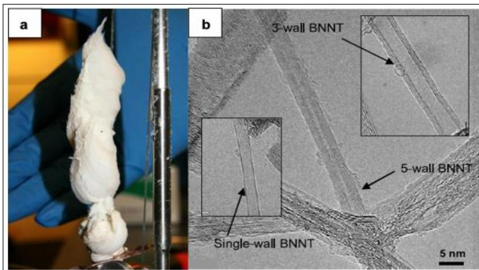
(a) 200 mg of BNNTs synthesized by the laser ablation method in a one production process. (b) TEM image of one-, three- and five-walled BNNTs. Source: M.W. Smith et al., Very long single- and few-walled boron nitride nanotubes via the pressurized vapor/condenser method. *Nanotechnology* 20(50), 505604 (2009)
